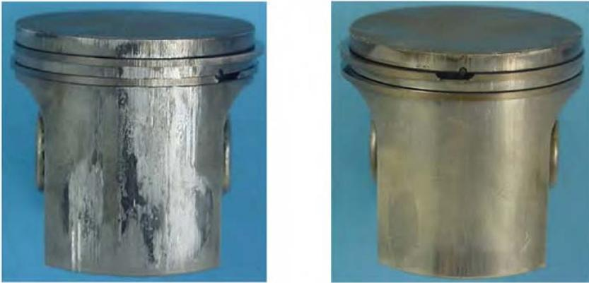
In the combustion chamber, lean is lean; it does not matter if air entered the engine somewhere other than the carb, leaning out the mixture, or if the fuel flow was restricted, leaning out the mixture. If the engine does not have a rev-limiter, lean running will cause over-revving. A saw with a lot of run time will get a polished, buffed appearance on the bottom of the intake skirt, but over-revving will advance this buffing effect considerably, as the picture on the right indicates.
