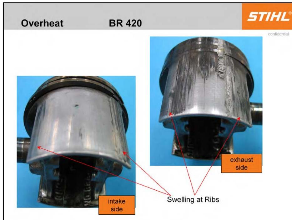
This is sometimes referred to as “4 point scoring”, implying that the piston swells at the four corners where the support webs for the skirt are located.
