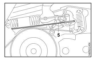
When the brake is off, the brake cable (5) must hang loosely, i.e. no tension, in the crankcase
