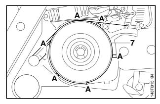
• The brake band (7) must locate snugly, i.e. no play, against the points (A) in the crankcase
