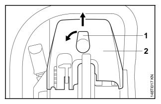
Release twist lock (1) and remove the carburetor box cover (2)
