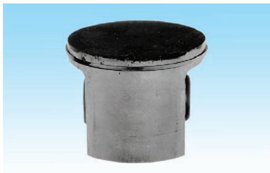
Small score marks and a matt, grey surface on the piston's inlet side caused by fine dust particles
