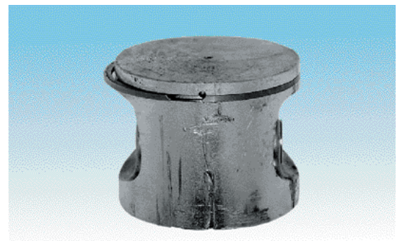
Irregular grooves on the piston's inlet side caused by a broken roller retainer
