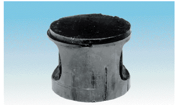
Deep, irregular grooves caused by a loose circlips is here shown here on the piston's inlet side
