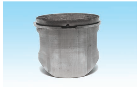
Piston from the inlet side with normal wear and normal discolouring
