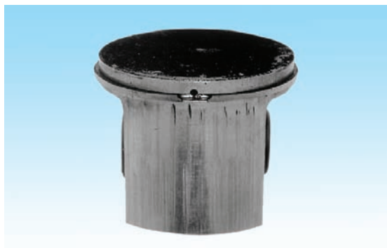
The piston scored and worn from the piston ring down on the inlet side
