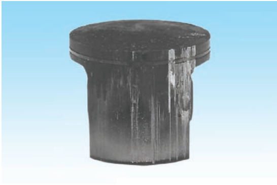
The piston ring (seen from the inlet side) is stuck in the groove and the dark discoloration under the piston ring is due to compression blow-by
