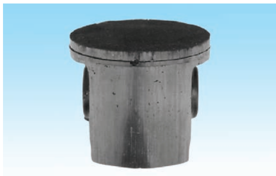
Particles of dust and dirt from carbon-like deposits on the top of the piston and in the piston ring groove
