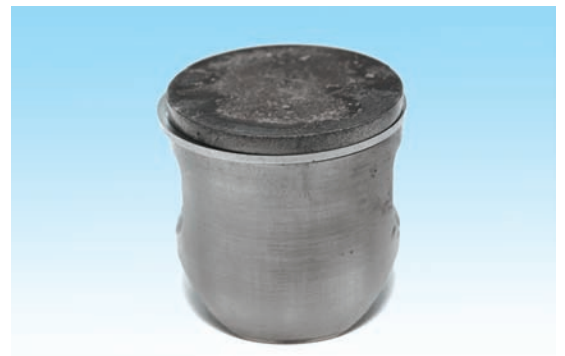
Piston from the exhaust side with normal wear and normal discolouring
