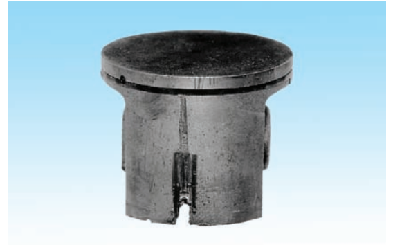
Extensive damage to the lower part of the piston's inlet side
