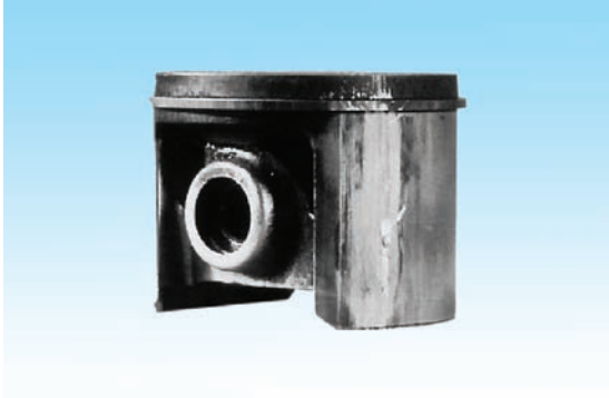
Small to medium scoring within the exhaust port area
