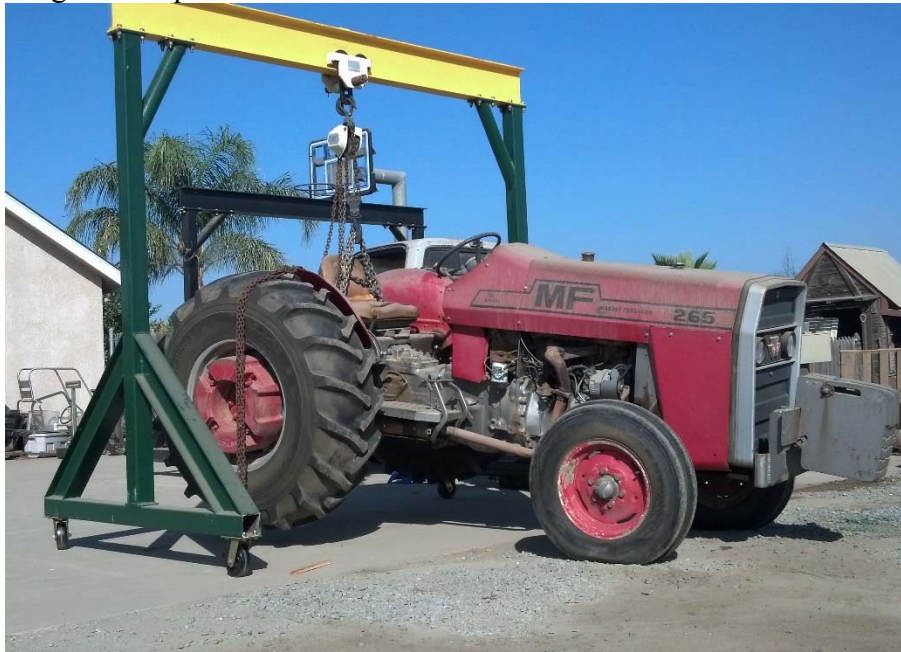
Figure 23. Tractor lifted and fully supported by hoist.
