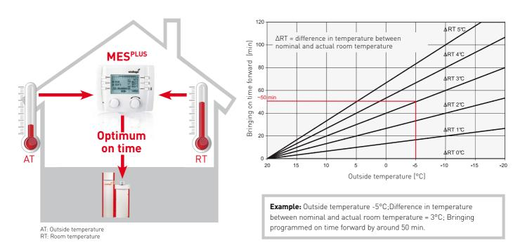
The fact that the system automatically works out the latest possible on time means that the system is operated efficiently without any loss of comfort because the room is not heated unnecessarily before heating is needed and heat from other sources, such as a stove or sunlight, is also taken into account.
