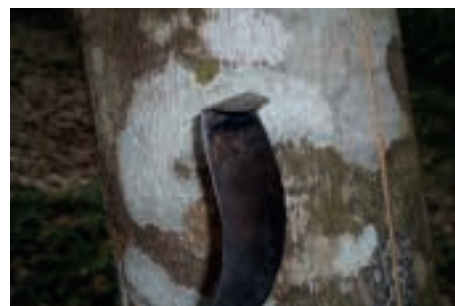
The business end of a rubber tapping knife; these are made locally from old vehicle suspension springs and are as sharp as a razor.
