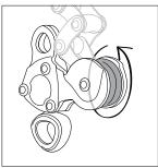
• Check the condition of the swivel (cracks, deformation, etc.).
