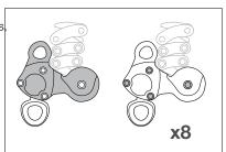
• Check the edges of the attachment hole for wear caused by connectors.
